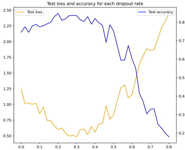
Figure 7.16: Dropout rate V.S. test loss and accuracy
