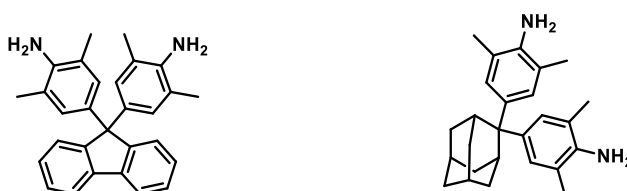
Figure 4.2: The structures of the two specifically designed diamines designed to prevent phthalocyanine stacking.
